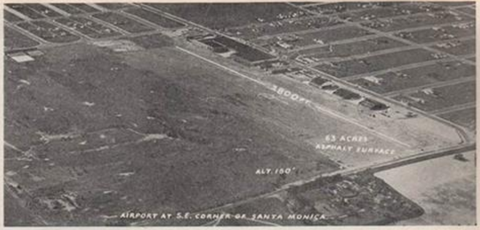
SANTA MONICA. — Clover, M. To SE. of city. Alt. 150 ft. Rectangular. 63 A., asphalt surface. Runways 3,000 by 200 ft., entire field available. Pole line, buildings, radio towers. N. Beacon, boundary, approach, obstruction, landing area flood lights. Beacon, rotating green. Service day and night. Left hand turns permitted in landing and taking off SE.; right hand turns in landing or taking off to E. or N.
