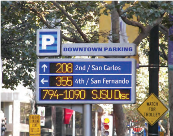
Parking signs in downtown San Jose display real-time availability for parking garages.
