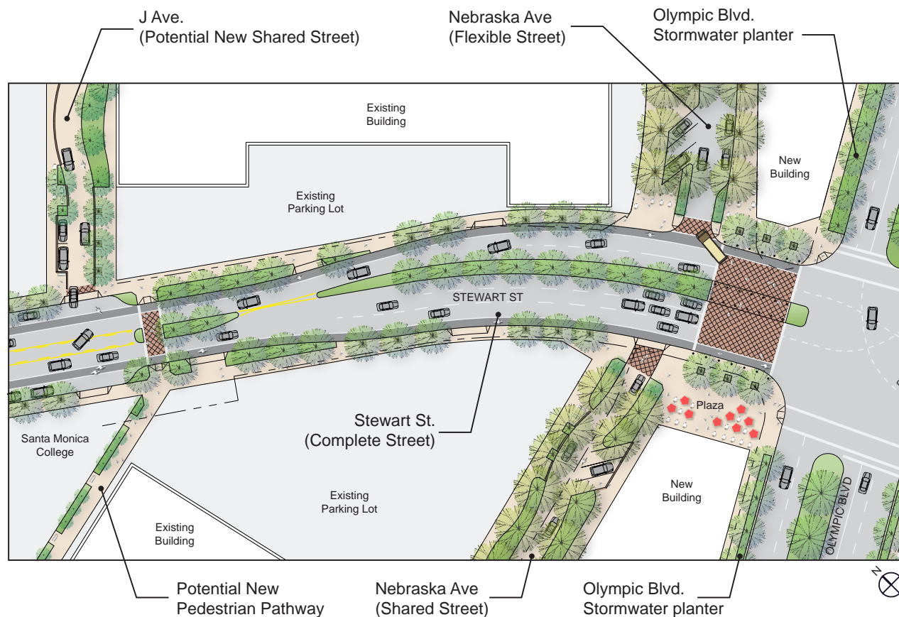
Figure 4.C.02 Proposed Street Improvements on Stewart Street at Olympic Blvd. and Nebraska Ave.
