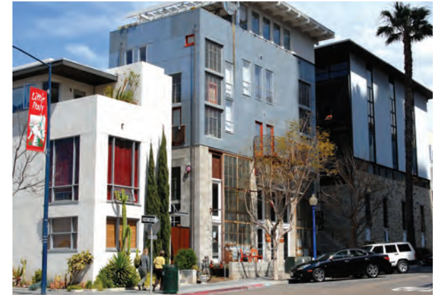
This streetscape exhibits distinct building height modulation that adds visual interest to the skyline.
