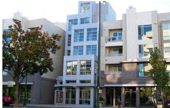
On corner sites, the residential lobby should be located on north/south streets, where practical leaving the east/west streets for uninterrupted storefronts.
