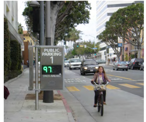
Real-time occupancy monitoring systems can be utilized in commercial and residential areas to effectively communicate parking availability to the public and to streamline the process of looking for parking.
