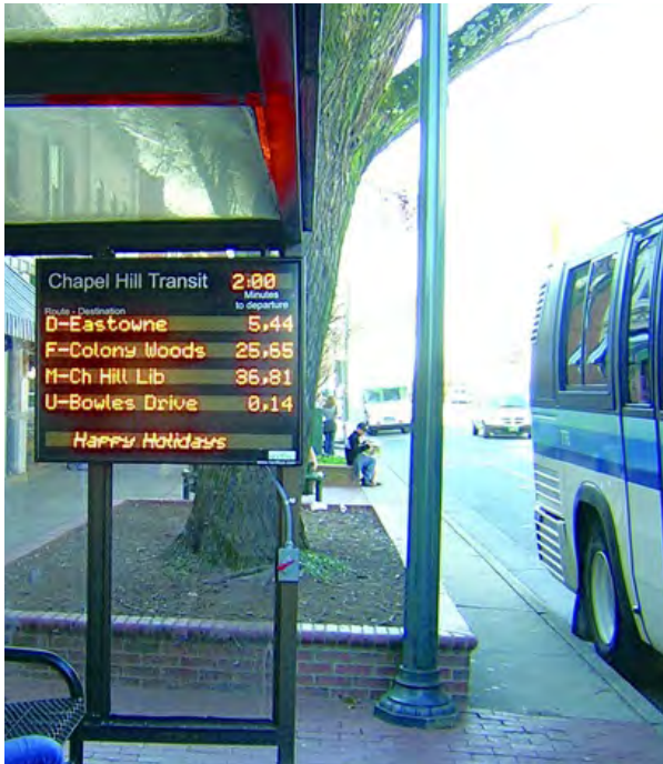
Transit investments that enhance passenger convenience could include bus shelters that provide real-time information such as time and next bus arrival.
