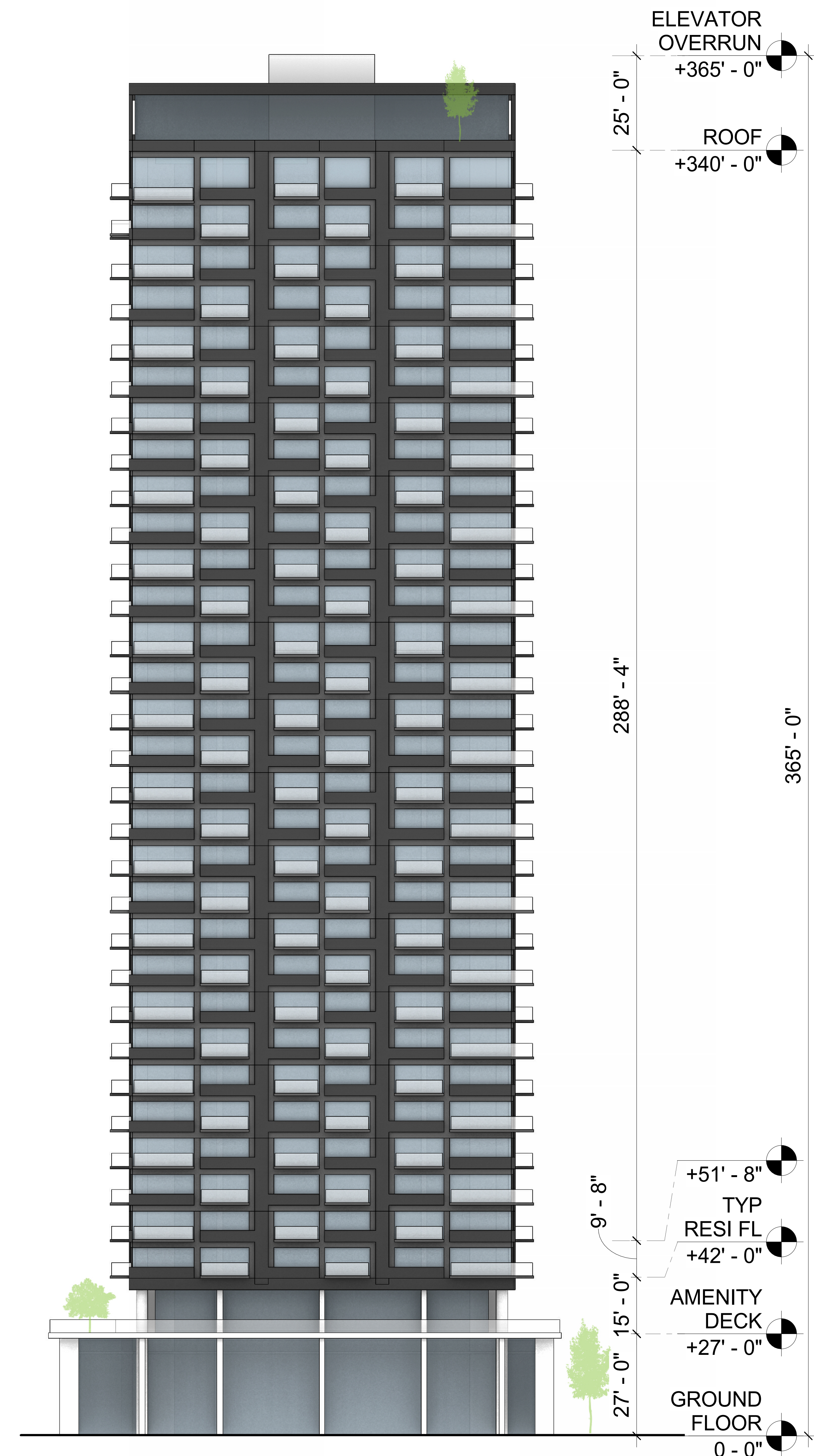
1 SB330 - SOUTH ELEVATION
