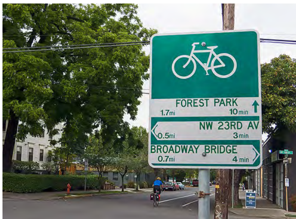
Bicycle wayfinding with destinations, distances, and approximate travel times. Source: Flickr user Richard Durdl, Creative Commons 2.0
