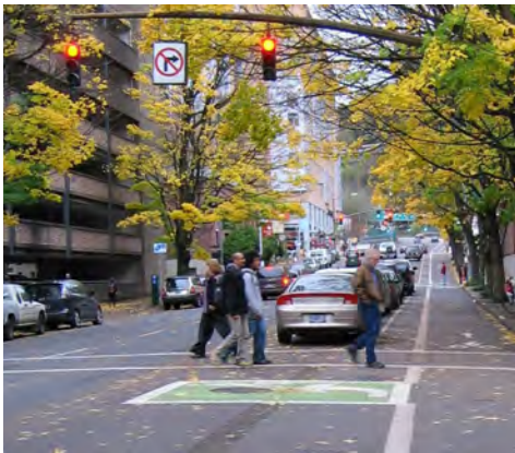
Left-turns off of cycle tracks can be facilitated by box turn facilities. Right turns off of connecting streets should be limited to the green phase only. Source: Nelson\Nygaard
