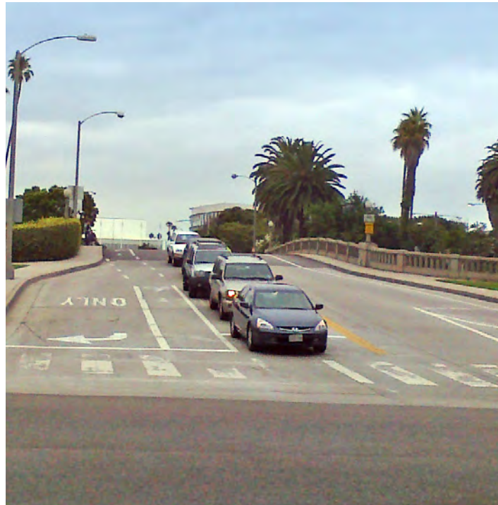
Left image: Right turn merge lane treatment where Main Street intersects with Colorado Avenue. The conflict zone between the dashes can be colored green for additional visibility. Right image: The MUTCD provides guidance on bike lane design at right turn lanes. Source: City of Santa Monica (left), MUTCD Figure 9-C4 (right)
