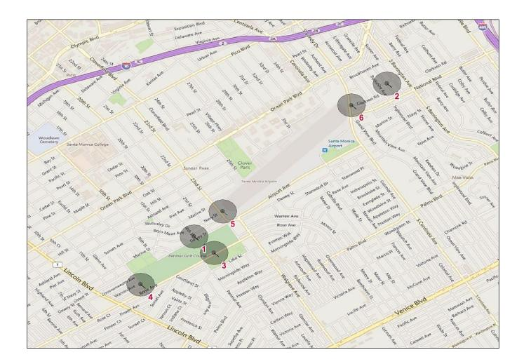
Note: ONLY Remote Monitoring Stations 1 & 2 are used for the Enforcement of the 95.0 dBA Single Event Noise Exposure Level (SENEL) maximum allowable noise level.
