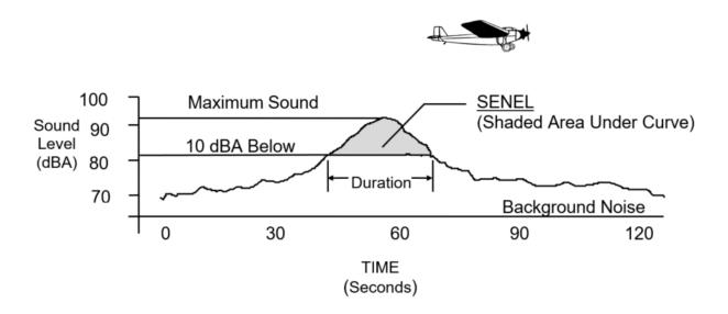
**A-WEIGHTED SOUND LEVEL (dBA)** – The sound pressure level in decibels as measured on a sound level meter using the A-Weighted filter network. The A-weighting filter de-emphasizes the very low and very high frequency components of the sound in a manner similar to the response of the human ear. It is a numerical method of rating human judgment of loudness.
