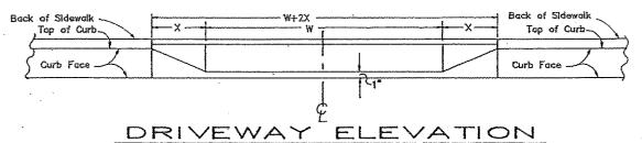
WHERE MAXIMUM SLOPES (10% ON RAMP AND 2% ON DEPRESSED SIDEWALK) CANNOT BE MET BECAUSE OF HIGH CURB OR NARROW SIDEWALK, DEPRESS BACK EDGE OF SIDEWALK UNTIL SAID SLOPES ARE OBTAINED, BUT THE LONGITUDINAL SIDEWALK SLOPES OUTSIDE THE LIMITS OF THE DRIVEWAY TO MEET THE DEPRESSED SIDEWALK SHALL BE NOT MORE THAN 6% GREATER THAN THE LONGITUDINAL SLOPE OF THE ADJACENT SIDEWALK.
