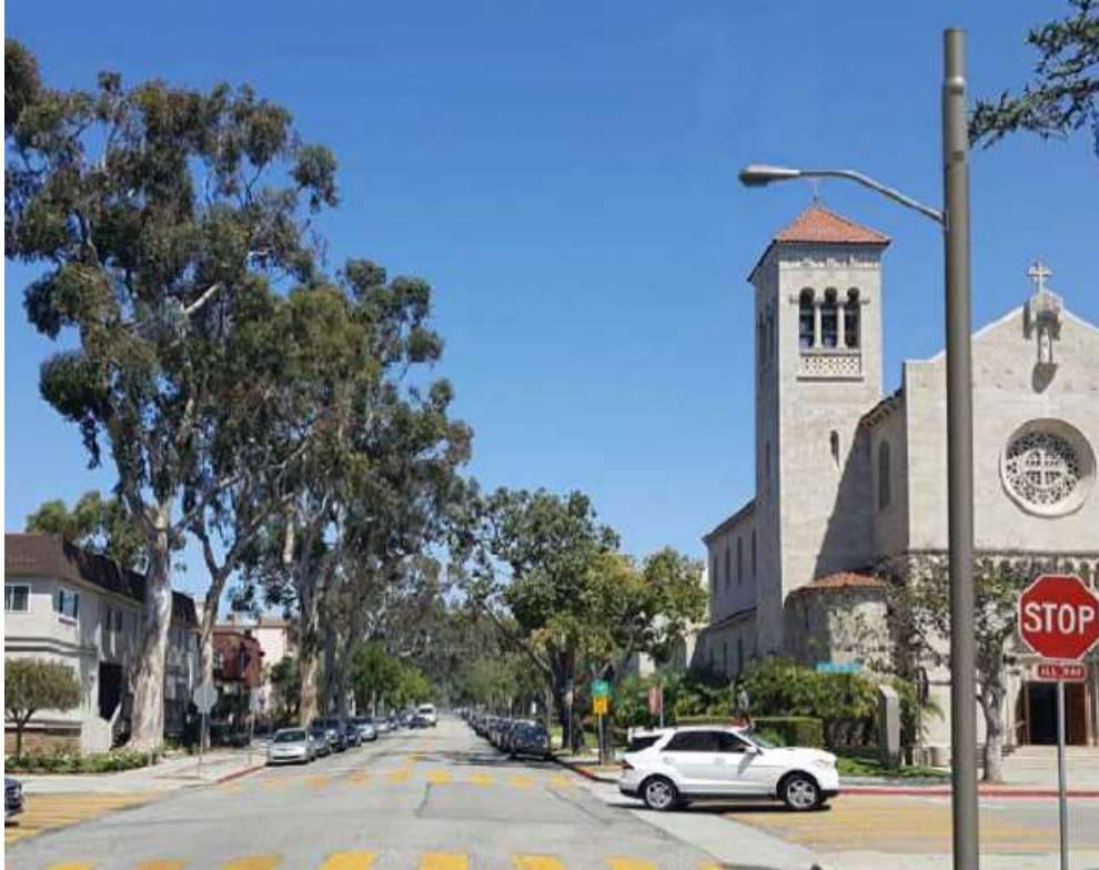
Figure 1: A photosimulation of a Southern California Edison streetlight with a personal wireless service facility located at the southeast corner of 7 th St and California Ave. The concealment shroud and cantenna meet the City's design standards. Other components, such as the WTR box, are installed below grade.
