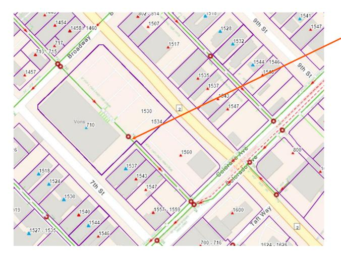
8-inch sewer line was relocated and increased to 12-inch sewer line by Developer based on increase in service required
